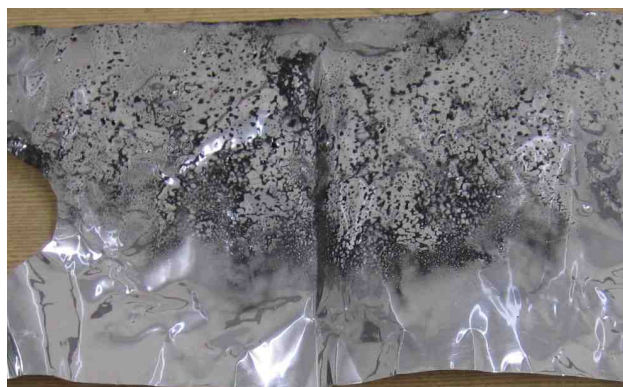
Fig. 3 A photograph of carbon soot deposited on the aluminum sheet set on the inner wall.
