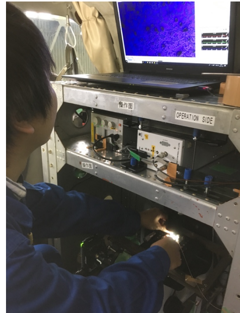
Fig.3 Experimental setup in a MU-300 rack. An inverted microscope was fixed on a vibration control device. Microscopic images were captured by the notebook computer set on the rack.
