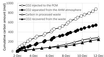
Fig. 3 Cumulative amount of carbon (mol) in  $CO_2$ injected to the PCM, separated from the AHM atmosphere and recovered from the waste and carbon in processed waste from December 2 to December 11 in the last experiment conducted in 2007.
