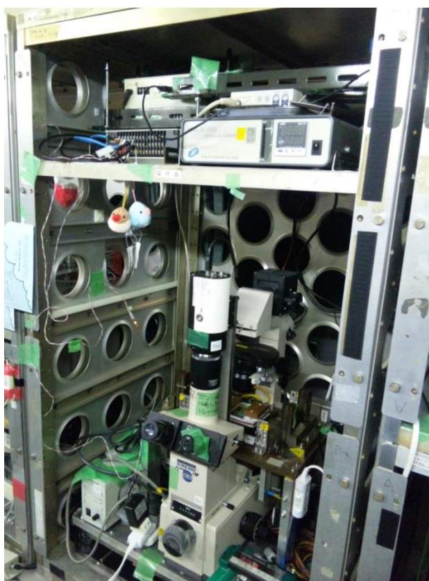
Fig.2. Experimental setup in G-II rack. An inverted microscope is fixed on a vibration control device. Precise focus adjustments during parabolic flights are achieved by using a piezo stage.
