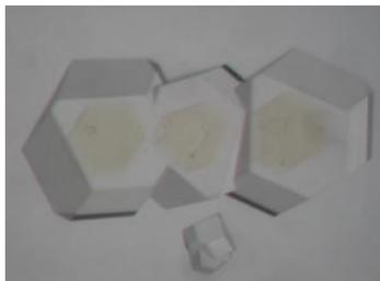
Fig.2. Regrowth of GI crystals (transparent part) on yellow chemically-fixed seed crystals.
