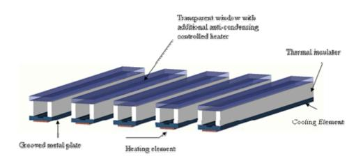
Figure 1: Typical layout with 5 model heat pipe cells
