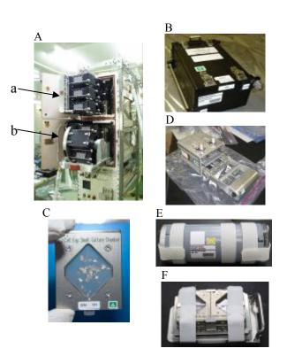
Fig. 2 Fish Scales Experiment hardware: CBEF (A) a microgravity section; "a", an artificial gravity section; "b"; MEU (B); Fish Scales culture chamber with scales (C); Pre-fixation Kit (E); Cell-fixation Kit (D); Sample holder assembly (F)
