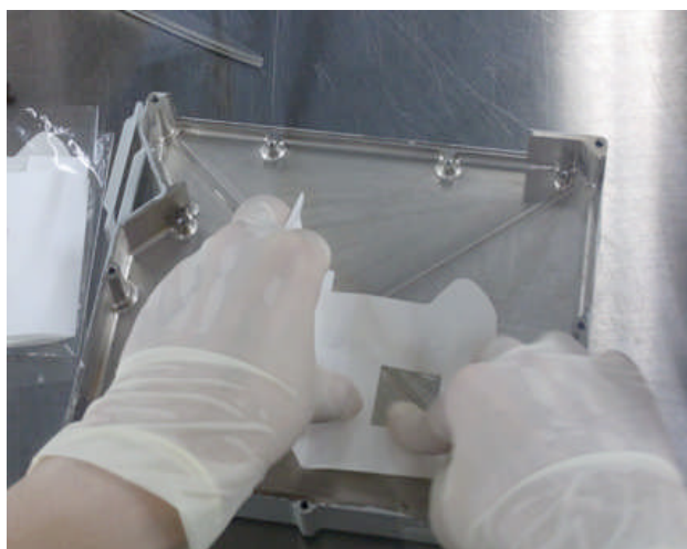
Fig. 2. Sampling of bacterial cells from MPC with microbe-collecting adhesive sheet.
