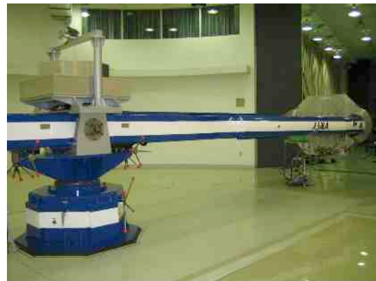
Fig. 1 Photo of the Rotation Acceleration Generator at JAXA Tsukuba Center.
