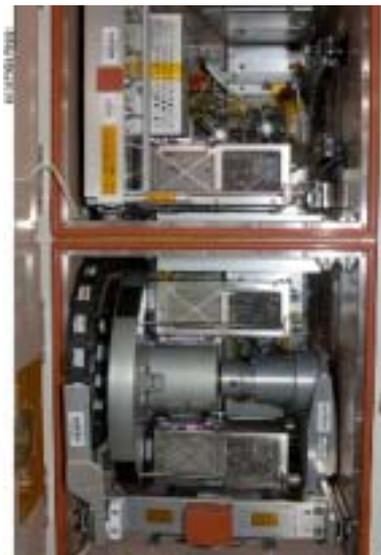
Figure 1 Plant Experiment Unit inside CBEF (Upper is micro gravity compartment, Lower is 1-G turn table)
