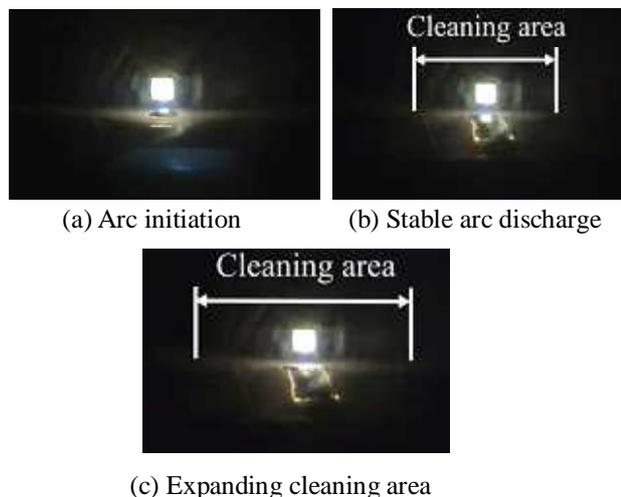
Fig. 4 AC arc discharge phenomena in vacuum
