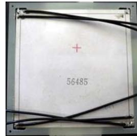
Fig.1. Arrangement of the electrodes on the surface of PZT element. The size is 40x40x1 mm<sup>3</sup> and the width of the four small electrodes is 2 mm.
