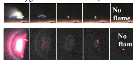
(b) No flame spreading, flow velocity  $U=0.03$  m/s, oxygen concentration  $X_{O_2}=8$  %
