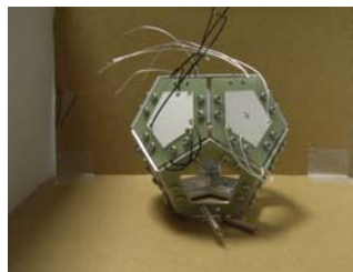
Fig.1. Frame of the dodecahedral detector.
