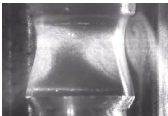
Fig.2 Visualization of thermocapillary convection and surrounding air motion
