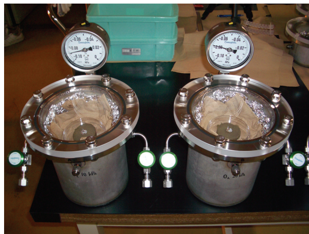
Fig.1 Vacuum vessels for rearing silkworm under low pressure.
