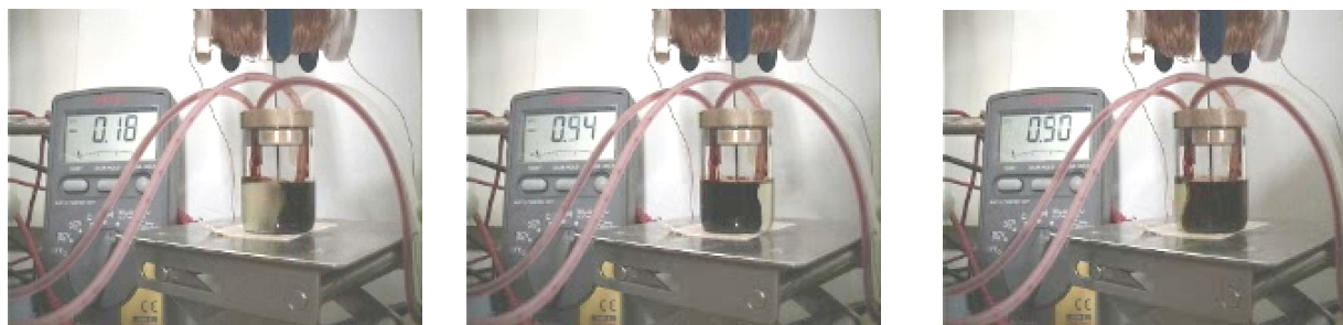
Fig. 6 Typical example of continuous rotation of half column of liquid pair by the supply of liquids
