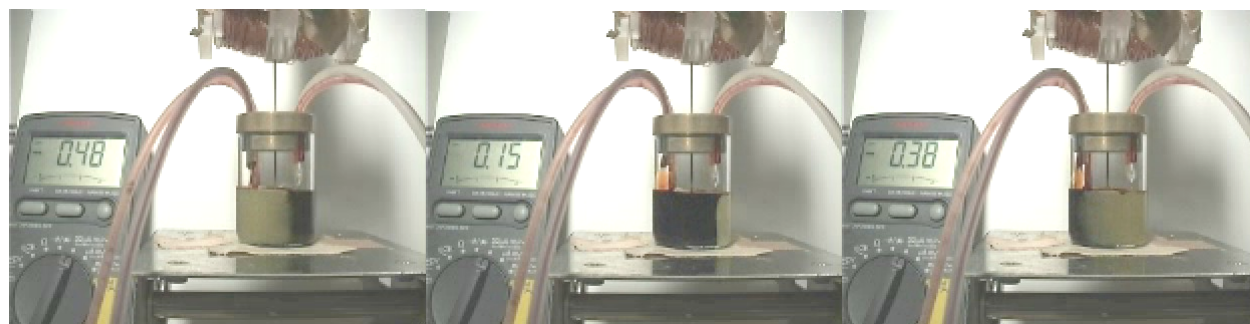
Fig.8 Recovery of rotational motion of half column of liquid pair by the addition of organic liquid waste
