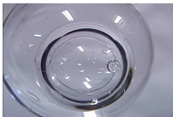
Figure 2 Small droplet does not coalesce with a surface of inner wall of a bubble. NASA Saturday morning science.
