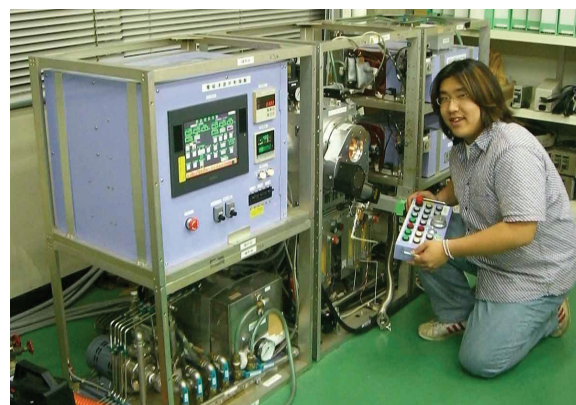
Fig. 4 航空機搭載用電磁浮遊装置：PFLEX: Parabolic Flight Levitation Experiment Facility.
