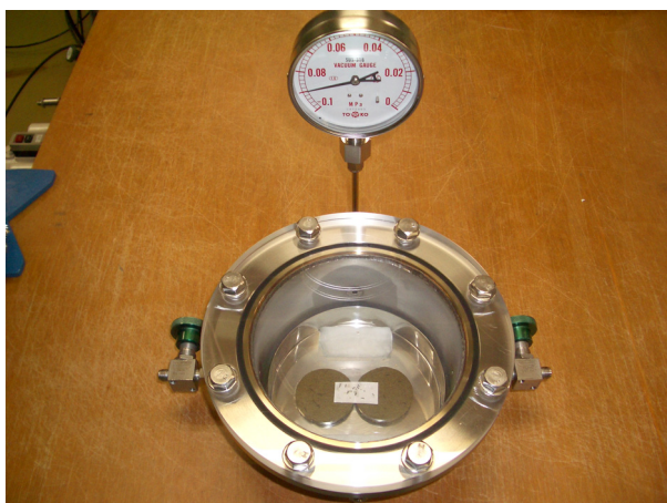
Fig.1 Vacuum vessel for breeding silkworm under low pressure.
