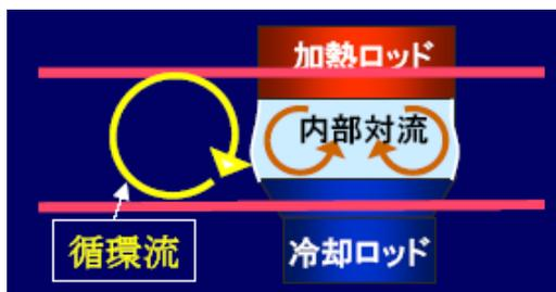
Fig.3 Partition disks to suppress the surrounding flow
