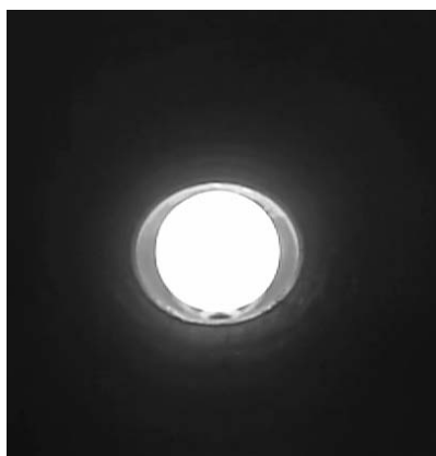
Fig. 2 Levitated liquid Zr_{70}Cu_{30} alloy sample with the diameter of about 2mm.
