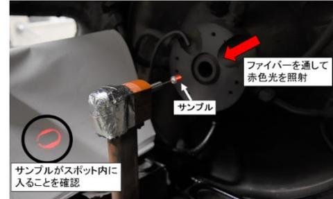
Fig. 2 Focusing lens setup (HR4000 spectrometer)
