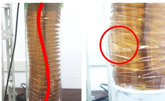
Fig.7 Deformation of inflatable tube
