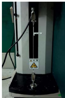
Fig. 2 Test apparatus for cyclic tensile test of a cable assembly
