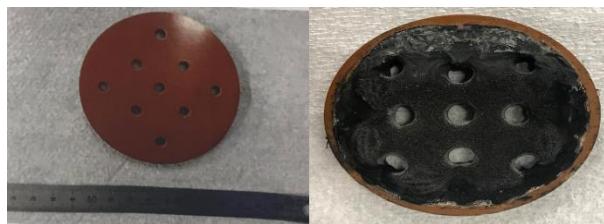
Fig.9 Appearance of baffle plate before and after burning (1)
