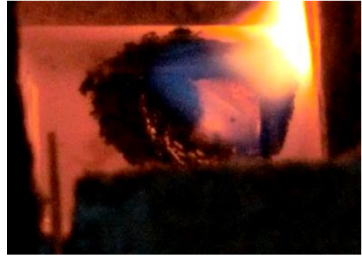
Figure 11 State of combustion flame (AN 5 mass%).
