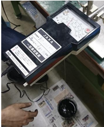
Figure 4 Shows the experiment using of analog-type visco tester.
