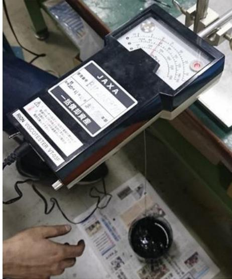
Fig.3 Shows the experiment using of analog-type visco tester
