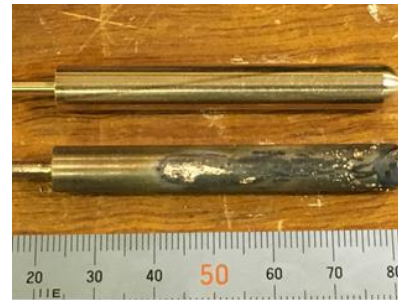
Figure 13 銅陽極の損耗
