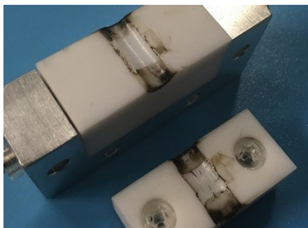
Fig. 11 Feature of the PTFE cavity after cleaning
