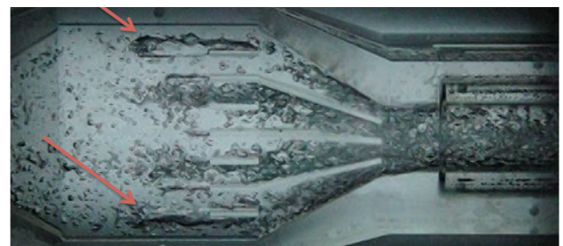
図 2.3 気泡の滞留 (G:1 [l/m], L:20 [l/m])
