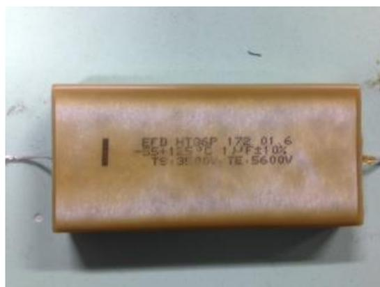
Fig. 4 Capacitor for  $V_c=1$  kV..
