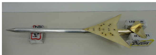
Fig.3 The wind-tunnel test model for the M2011 baseline configuration.
