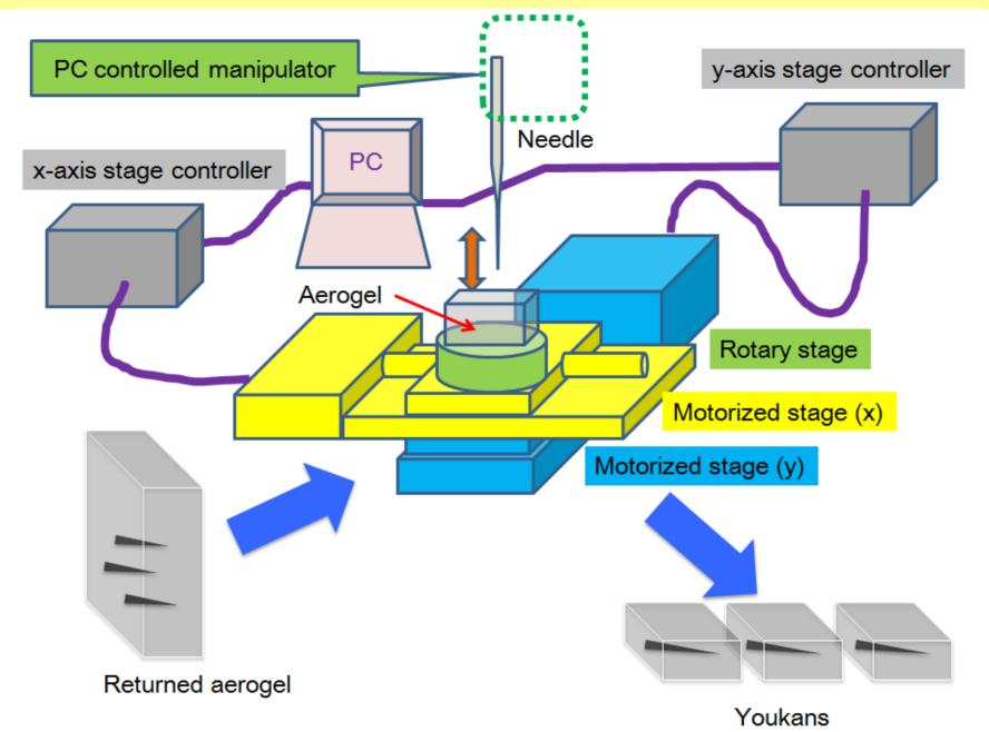
Fig. 2 Youkan machine. A returned aerogel will be separated into several Youkans and offered to analyses.
