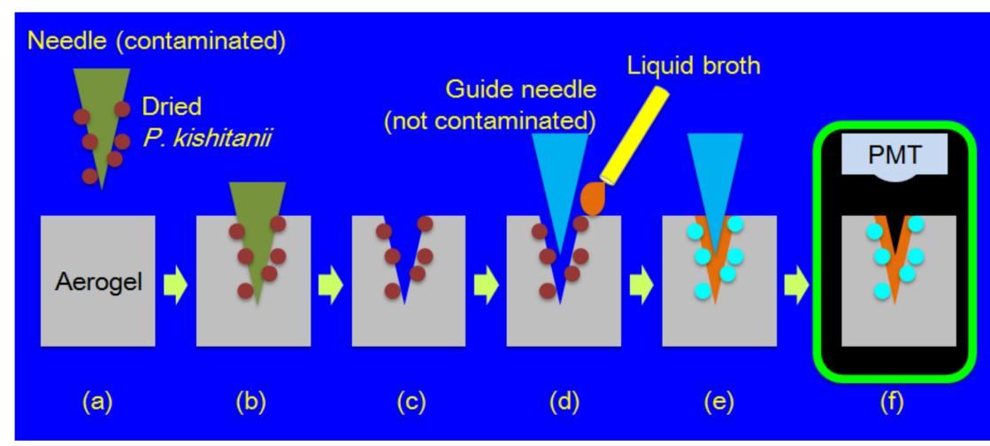
Fig. 8 Experimental procesure. Firstly, dried *P. kishitanii* cells were attached on the needle surface (a). The needle was carefully inserted into an aerogel (0.01 g cm<sup>-3</sup>) (b). After the removal of the needle (c), a guide needle was placed into the hole (d) and 2-3 μL of liquid broth (marine broth) was added (e). Luminescence intensity from the P. kishitanii attached aerogel was measured using a luminometer (Lumicounter 200; Microtech Co., Funabashi, Japan) (f).
