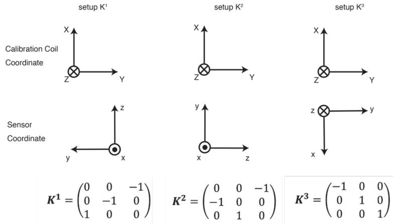
Fig. 2. Configurations of the coil and the sensor
