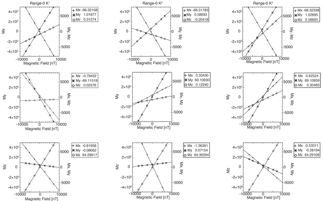
Fig.3 Output M relative to the applied magnetic field B within 8000-nT range
