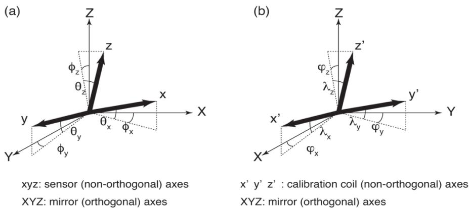
Fig. 1. Definitions of the angle (a) MGF-S and sensor mirror coordinates (b) calibration coil and coil mirror coordinates
