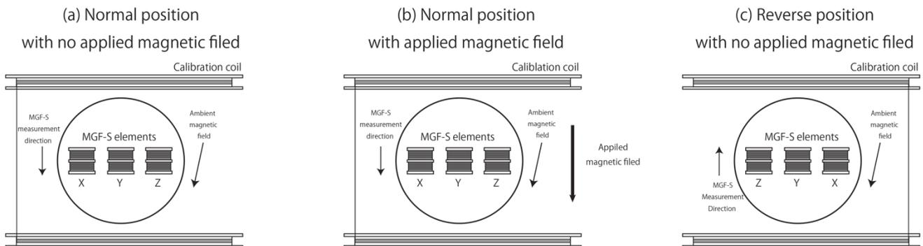
Fig 4. Each position of the MGF-S in the temperature experiments
