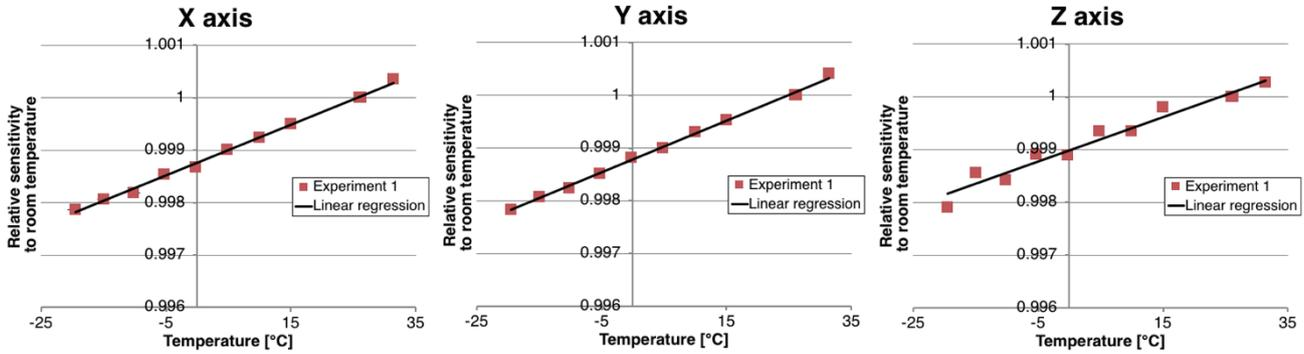
Fig. 5. Temperature dependence of sensitivity. Ratio to the sensitivity to the room temperature 26.1 °C is shown
