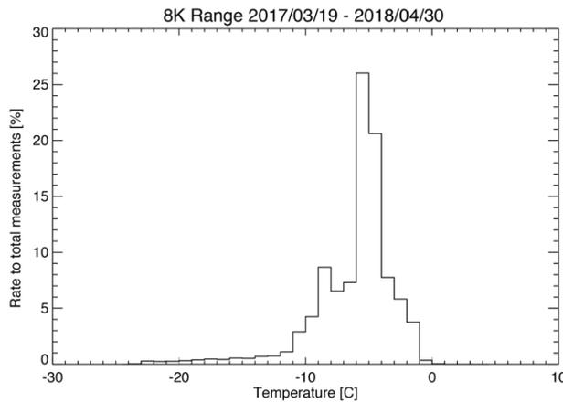
Fig. 6. Histogram of the rate of total measurements of MGF 8000-nT range between March 19, 2017 and April 30, 2018
