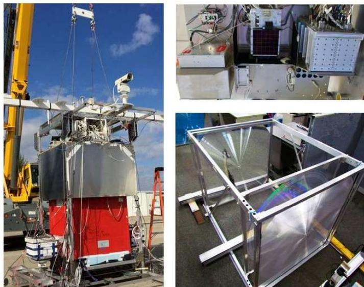
Figure 3: Left: The EUSO-SPB payload in the flight configuration during standalone hang tests in Palestine, Texas. Top right: the electronics with the PDM focal surface in the centre. Bottom right: the Fresnel lens optics.
