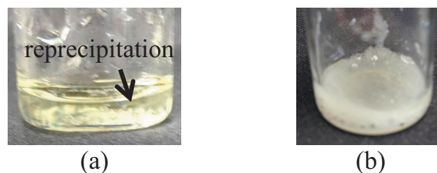
Fig.4 (a) ADN/AA=6/4 mixture after heating at room temperature (b) ADN/AA=7/3 mixture with impact
