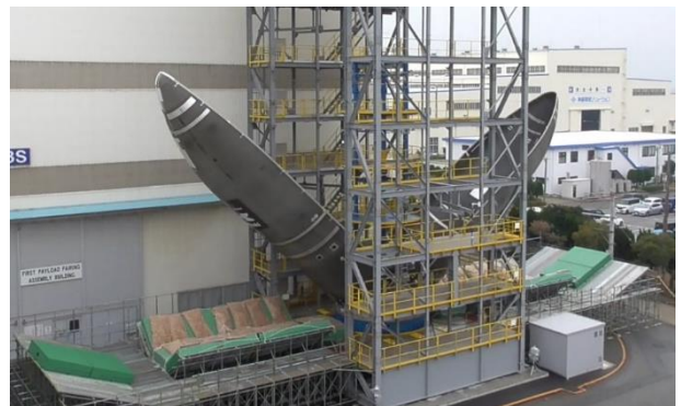
Fig. 6 Fairing separation test
