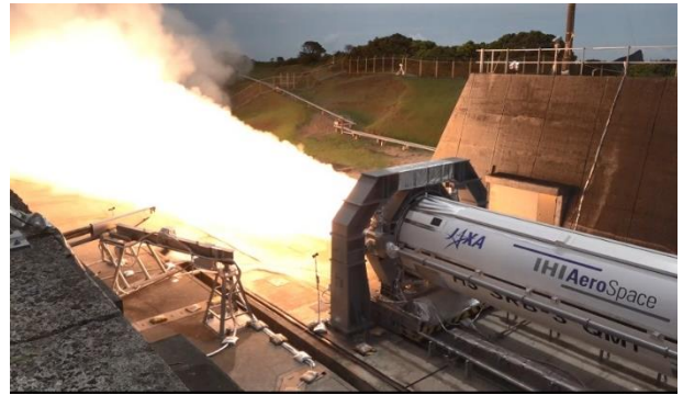
Fig. 5 SRB-3 Firing Test
