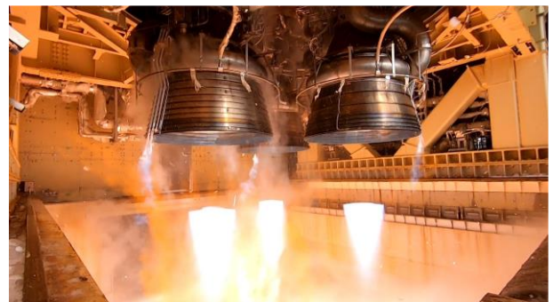
Fig. 8 First stage battleship firing test
