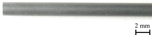
Fig. 4 Silicon carbide (SiC, diameter 2.0 mm)
