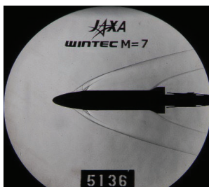
Schlieren Photo 1/8 Model
