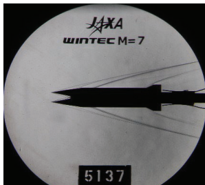
Schlieren Photo 1/8 Model
