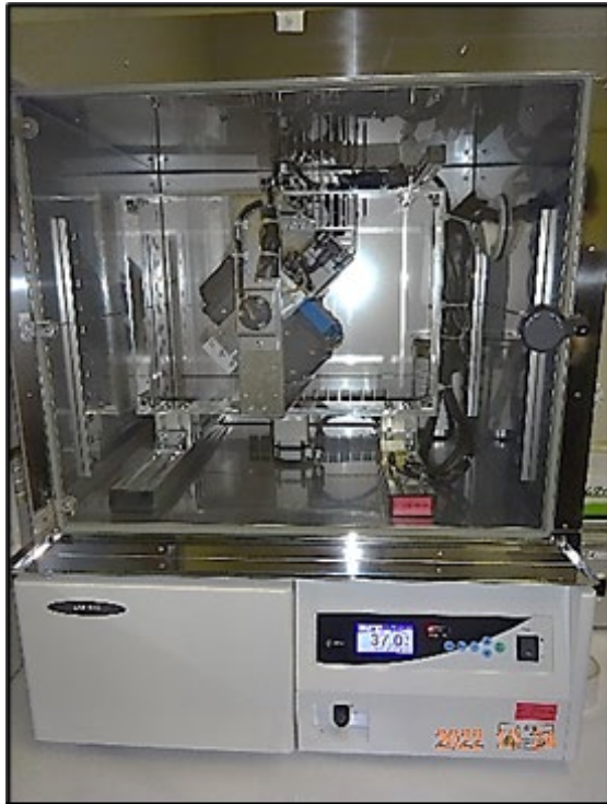
Fig.2 Photograph of Simulator of the environments on the Moon and Mars with Neutron-irradiation and Gravity-change (SwiNG).
