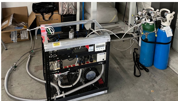
Fig. 3. The ground vacuum system with four high-pressure gas cylinders.
