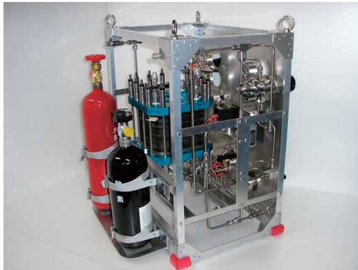
Figure 2. A photograph of a fuel cell stack and a gas distribution subsystem.
