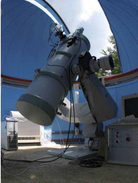
Figure 4: The telescope (35cm Newtonian telescope \epsilon 350N manufactured by Takahashi Co. Ltd.) and the camera (2K \times 2K back-illuminated CCD camera FCC-104B manufactured by N.I.L. Co. Ltd.) used for the observation.
