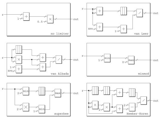
Fig. 5 Implemented flux limiter functions.
