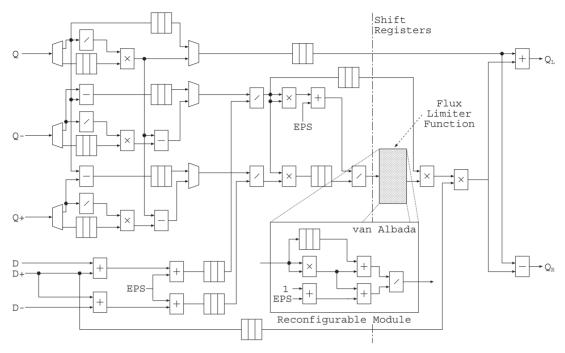
Fig. 4 MUSCL pipeline with van Albada limiter function.
