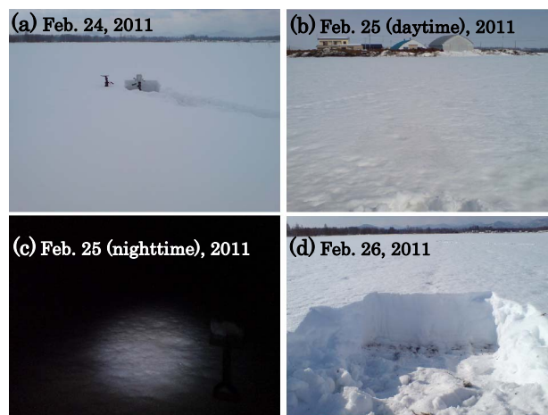
Fig. 2. Visible image photographs of snow covers taken at a snowfield in Hokkaido, Japan, on (a) Feb. 24 (surface snow type: partly rounded particles and faceted particles; air temperature: -5 to 0^\circ\text{C} ), (b) daytime on Feb. 25 (granular snow and patches of sun crust, 3^\circ\text{C}\text{--}5^\circ\text{C} ), (c) nighttime on Feb. 25 (granular snow and fragments of sun crust, -8 to -4^\circ\text{C} ), and (d) Feb. 26, 2011 (granular snow, -8 to -4^\circ\text{C} ).
