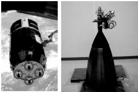
Fig. 1 “Kounotori” 3rd (HTV-3) and its thrusters. Thrust level is 490N class.
