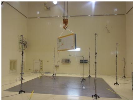
Fig. 9 Test configuration in reverberant chamber
