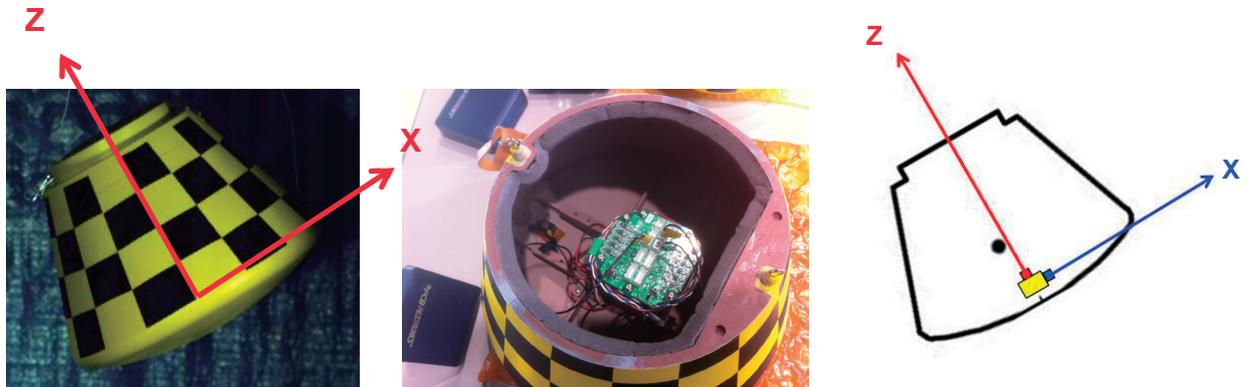
Fig. 8. 6.8% scale model of HRV for the water landing test
